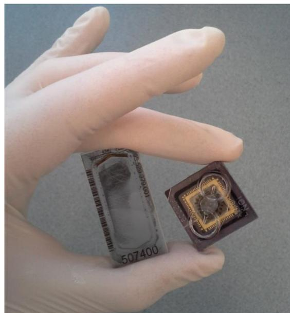
**Fig. IV/11. Picotiter plate and semiconductor chip used for next-generation DNA sequencing**
