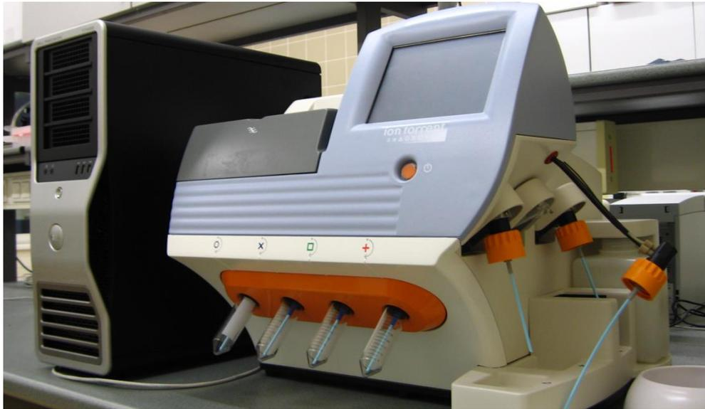
**Fig. IV/9.** The Ion Torrent PGM™ (Life Technologies) next-generation DNA sequencing system
