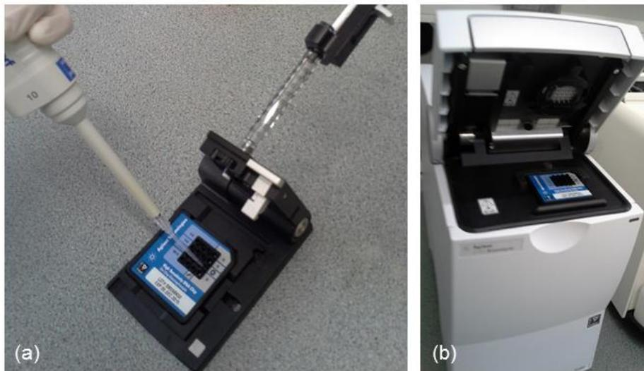
**Fig. IV/2.a-b The Agilent 2100 Bioanalyzer on-chip electrophoresis system**
