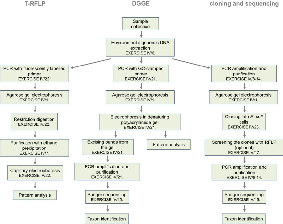
**Fig. IV/22. General process workflow of T-RFLP-, DGGE- and cloning and sequencing-based environmental microbiological studies**
