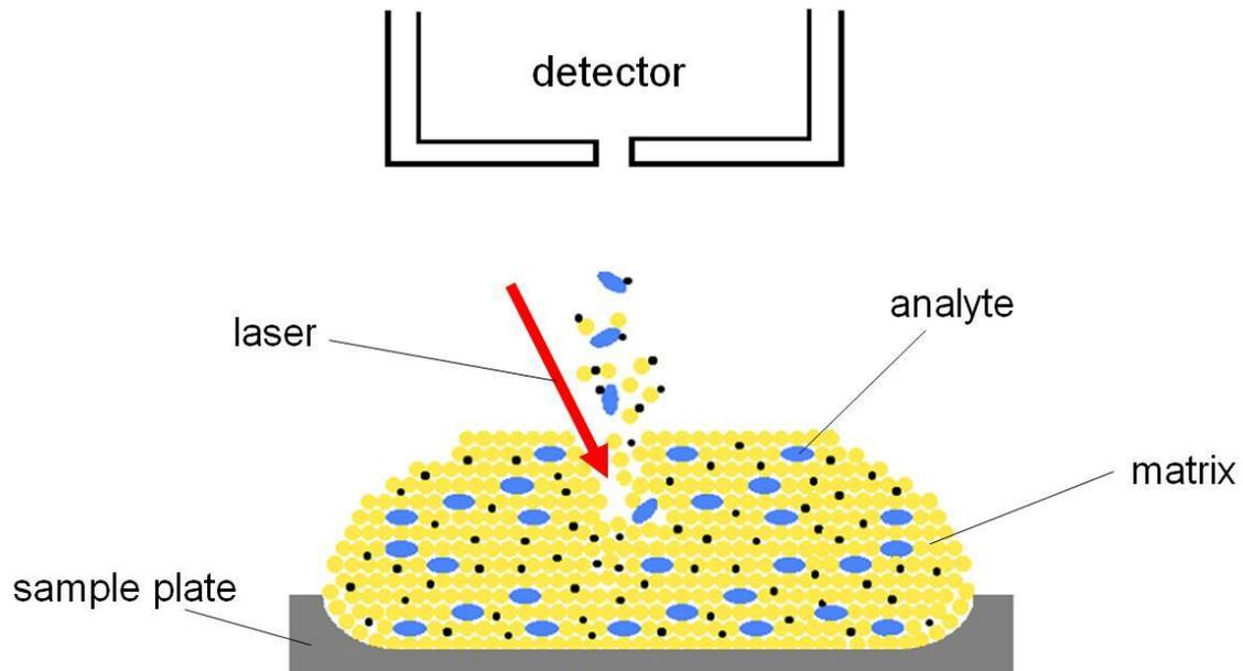
**Fig. III/7. Basic principle of MALDI**
