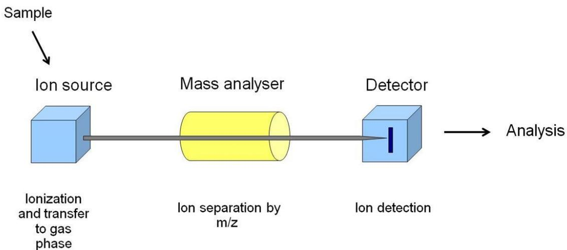
**Fig. III/6. Principle of mass spectrometry**
