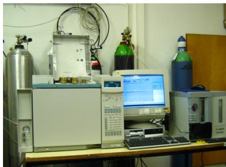
Figure 15.7: Gas chromatograph for greenhouse gas measurement at Hegyhátsál station, Hungary
