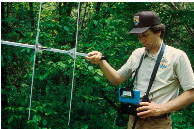
Figure XIX.1. main parts of the radiotelemetric equipment: a/ radio collar attached to the animal, b/. reciever with attached Yagi antenna
