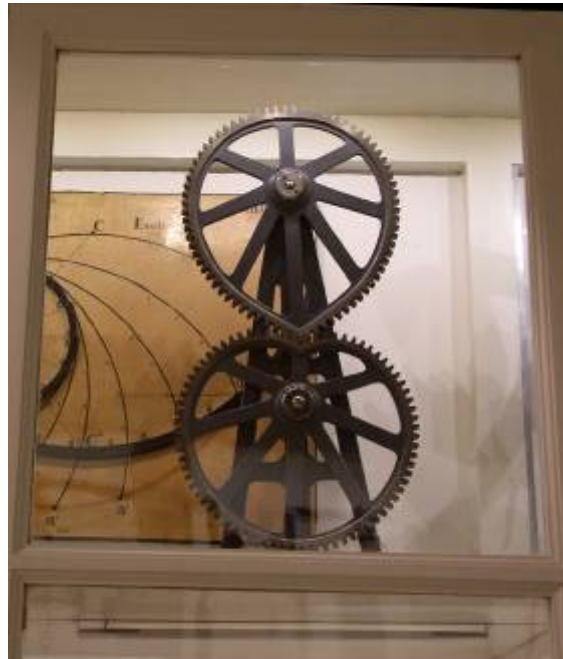
4.32. picture: Two cog wheels with peculiar shapes that set each other in motion. Istituto e Museo di Storia della Scienza, Florence. (Photo: Tamás Vásárhelyi.)
