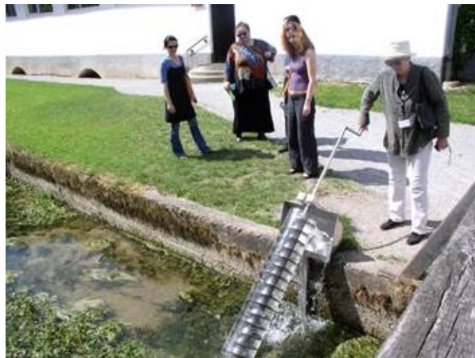
5.23. picture: An easy-to-realise, still much preferred by visitors interactive installation type is the water-powered machine. Here, a model of the Screw of Archimedes is put to use to upraise water from a creek near the museum building. The museum environment is utilised here to create a very natural and effective installation. (Photo: Tamás Vásárhelyi)
