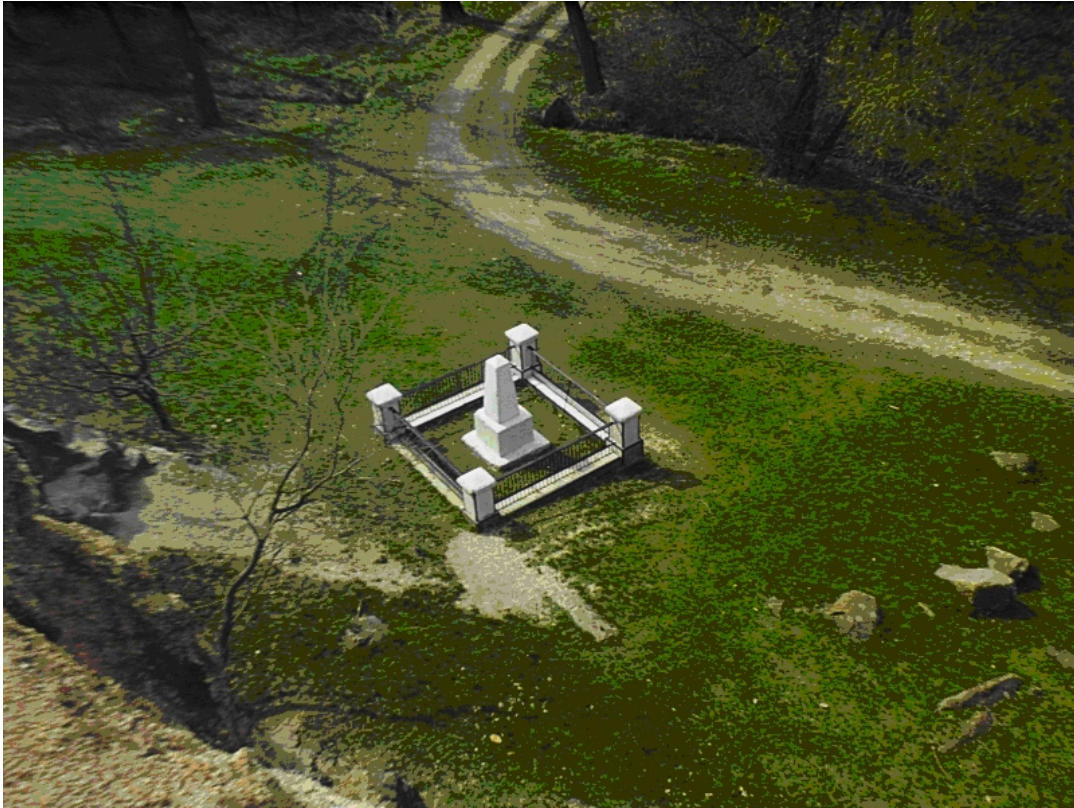
Fig. 43. The new point at Nadap (in the middle) and the old point's location at the hillside (on the left), the fundamental point of the Hungarian elevation network (Gy. Busics, 2012).
