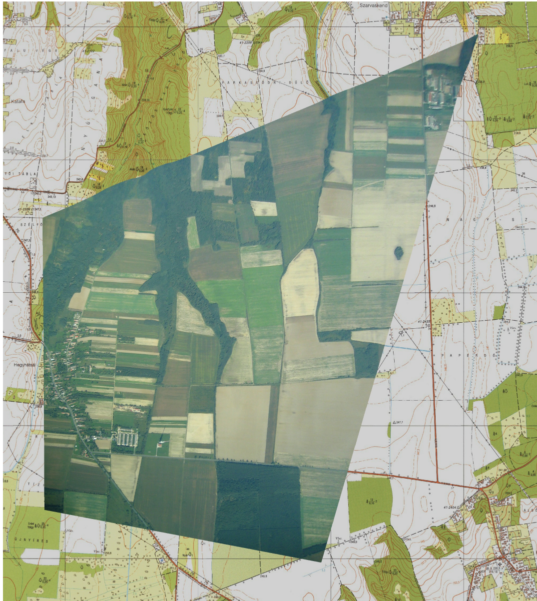
Fig. 58. Rectified version of the above photograph. The optical axis is far from the nadir direction, that's why the strange shape – however the fitting is good even in the far corner.
