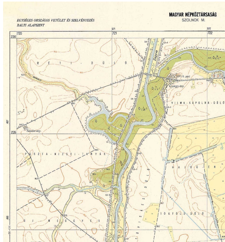
Fig. 25. Map sheet in Hungarian national grid without latitudes or longitudes indicated: the sheet boundary follows the projection lines.
