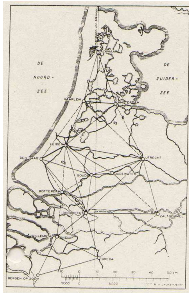
Fig. 12. The distance between the towns of Alkmaar (in the north) and Breda (in the south) was determined by the 1615 triangulation of Snellius, throughout swamps, marshlands and rivers.
