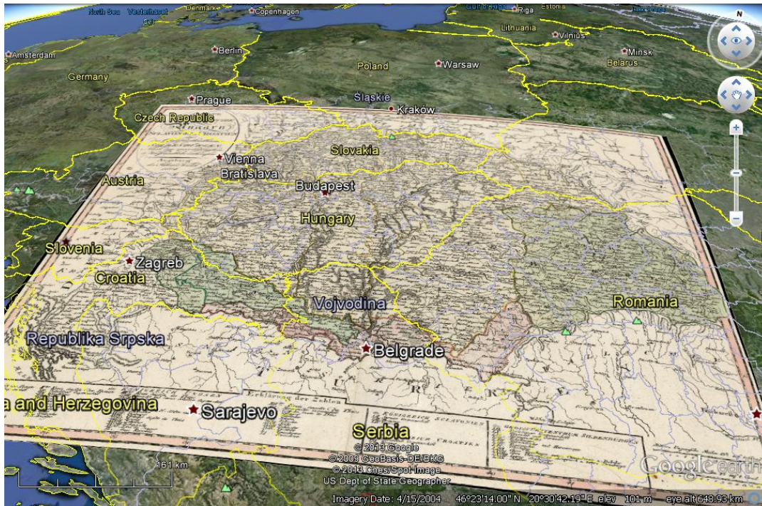
Fig. 1. The map of Hungary of Goetz & Probst from 1804 as a Google Earth layer: integration of completely different data technologies by the geo-reference.
