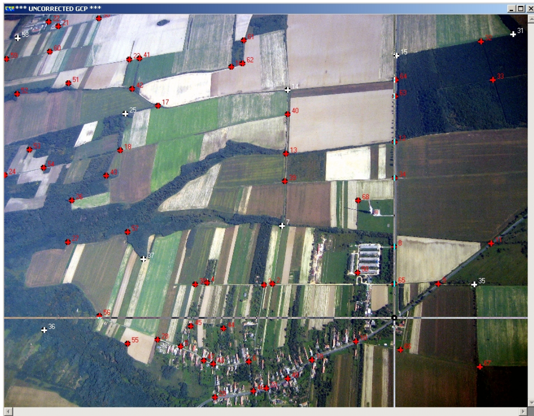
Fig. 55. GCPs in ortho-rectification: it is quite a work to find the best ones.
