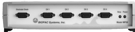
Figure 3.1. MP30 data acquisition unit. The device is connected to the computer by USB cable.
