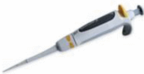
Figure 4.3. Automated pipette with adjustable volume. Yellow colour indicates a volume between 2-20 \mu\text{l} , while grey coloured pipettes can be used between 100 to 1000 \mu\text{l} .
