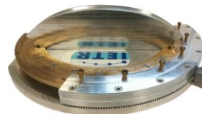
Steerable QO Radiator, Ka band, Groove Gap WG Feed, \pm 60^\circ
